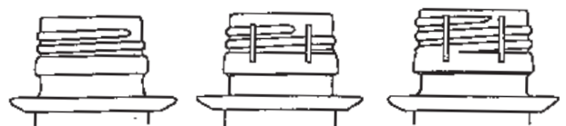
1. Screw thread replica of the glass bottle finish
